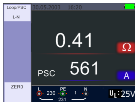
L - N Line Impedance – Measurement completed
