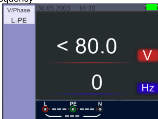
Standby screen for the Voltage and Frequency
